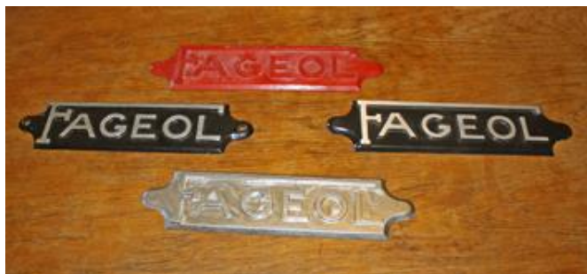
The pattern, an original name plate on left, and two new name plates
