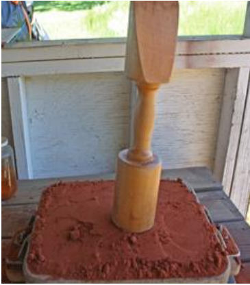
Sand has been riddled over the pattern and then rammed
