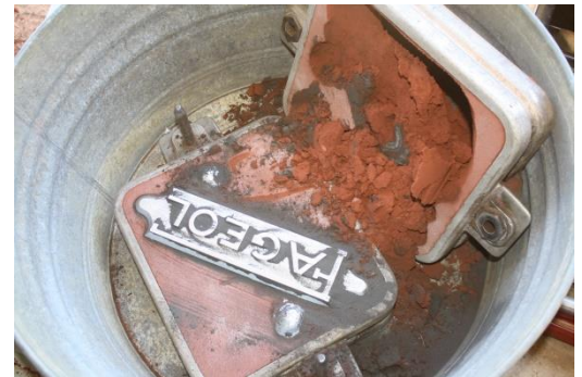
The mold has been poured and allowed to cool, showing the as cast name plate
