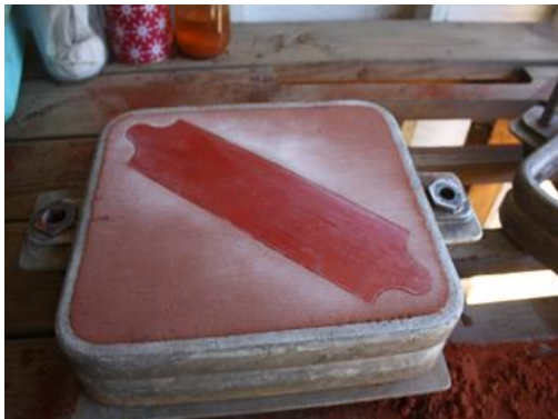
The mold is rolled over showing the pattern
