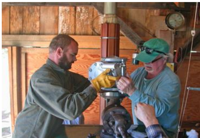
Lower right: Tom and Bill hoist the heavy steam-water separator
