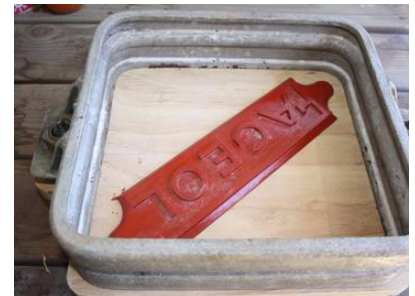
The pattern is laid inside the bottom of the flask--the drag
